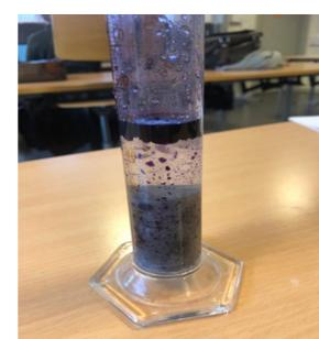
Fig. 3: Extraction of oil from chalk cores
