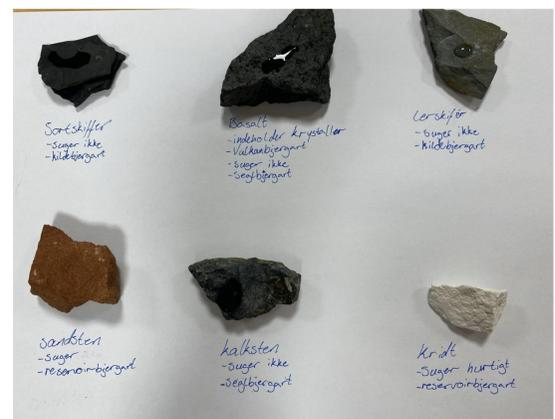
Fig. 1: Different rocks that are important for the formation and extraction of gas and oil.
