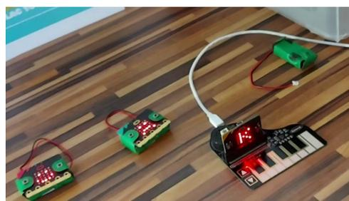
Robots do not crash, they use ultrasonic sensor to identify locations of surrounding objects. Robots – cheerleader waits for the winning car.
